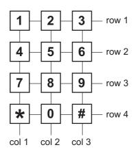
Almost all keypads, including computer keyboards, do not consist of individual switches, but are made up of a 'matrix' of switches in structured rows and columns. This is to reduce the number of interfacing lines required – a 12 key keypad only needs 7 interfacing lines (4 rows + 3 columns) as shown left. At first this can make the interfacing of a keypad seem daunting, but once you understand the 'scanning' process it can be seen that the actual electronic circuit is very simple.
