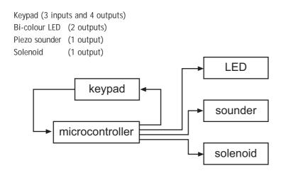
When using a keypad, it is important to have some feedback to the user to acknowledge that a key has been pressed. Commonly this is achieved with a buzzer or sounder, and so in this project we will use a piezo-sounder. In microcontroller projects a piezo-sounder is always preferable to a buzzer as it is low cost, it can be directly connected without any interfacing circuits, and can be used to produce a variety of different sounds.
