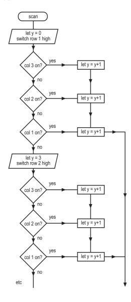
As soon as a hit is recorded, scanning ceases and a 'beep' sound is generated to create audible user feedback. The value of Y can then be tested against the PIN number to see if it is the correct value.
