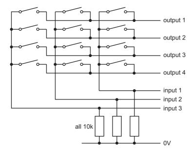
When no switches are pressed, there is no electrical connection between any row or column. Therefore all the inputs are at the logic level 0 (0V) status, as they are 'pulled low' by the 10k resistors connected to these lines. This means the input signal to the controller is 0-0-0 along the three input lines.
