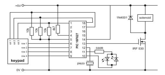
For clarity the PICAXE-18 download circuit (22k resistor and stereo socket) is not shown - see PICAXE manual for further details. 10k resistors are provided in SIL format to reduce pcb size.
