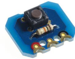
The following program tests the operation of the push button by lighting the an LED on the motherboard B.3 when the button is pushed.
