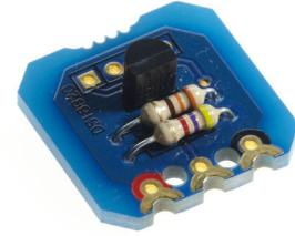
*The optional 4 way connector is for connecting an iButton probe, part RSA001 (not supplied).*
