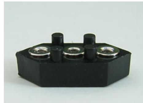
Note that the posts only allow the bric to be connected in one way. When correctly oriented the connecting bric will fit flush to the circuit board. If incorrectly fitted the connecting bric will be angled to the circuit board; in this case remove the connecting bric, rotate it through 180 degrees and then refit.
