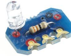
To check the IR Transmitters are working fully you will need two Microbots, one sending and one receiving and reporting what it has received. The operation of the IR transmitters is invisible to the human eye but can usually be observed by using a PC webcam, mobile phone camera or camcorder.
