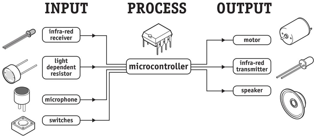
The electronic system that controls the Furby toy can be drawn as a 'block diagram'. The light sensor, microphone and switches all provide information to the microcontroller, and so these are known as 'inputs'. The microcontroller then 'decides' how to behave and may then operate the outputs e.g. make the motor move or generate a sound with the speaker. If another Furby is nearby they can 'communicate' by infra-red signals transmitted, and received, by the microcontroller.
