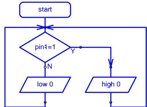
This program will switch output 0 on and off according to the light level.
