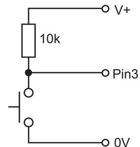
This layout is a little confusing, as it means that when the switch is pushed down, the logic level is '0'. When the switch is not pushed the logic level is '1'. This is known as an 'active-low' switch. In this project this is necessary for compatibility with the optional infra-red upgrade kit.
