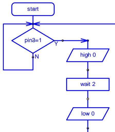
The LED on output 0 should light whenever the switch is pushed. If it does not check that the switch and 10k resistors are correctly soldered.
