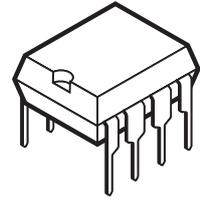
Microcontrollers are purchased 'blank' and then programmed with a specific control program. Once programmed the microcontroller is built into a product to make the product more intelligent and easier to use.
