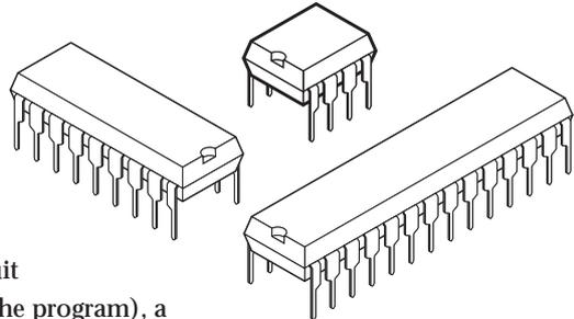
The microcontroller is an integrated circuit ("chip") that contains memory (to store the program), a processor (to process and carry out the program) and input/output pins (to connect switches, sensors and output devices like motors).
