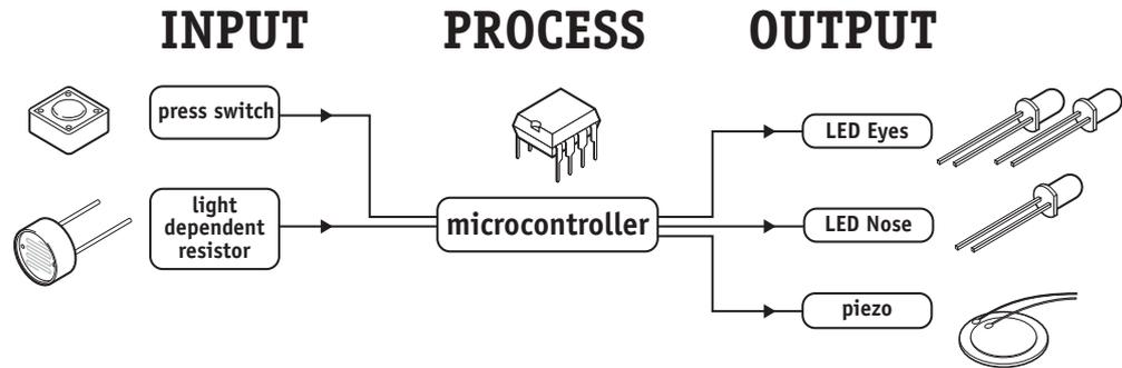
The electronic block diagram is shown below.
