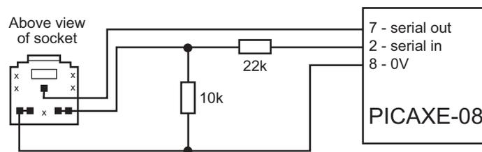
The socket and interfacing circuit is included on every PCB designed to be used with the PICAXE-08M microcontroller. This enables the PICAXE microcontroller to be re-programmed without removing the chip from the PCB - simply connect the cable whenever you want to download a new program!
