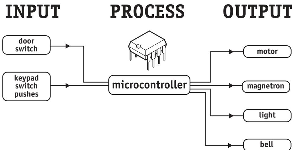
The program for the microcontroller is developed (and tested) on the computer and then downloaded into the microcontroller. Once the program is in the microcontroller it starts to 'run' and carries out the instructions.
