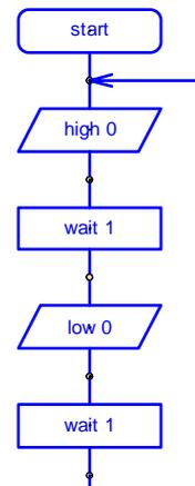
The nose LED should flicker as the program downloads. After the download is complete the LED should flash on and off every second. If the LED does not flash check that it is around the correct way and that the 330R resistors are in the correct positions on the PCB.
