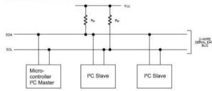
Note that more slave chips can be connected to the SDA and SCL lines, normally Rp has a value of 1kOHM. The clock generated by the master is called Serial Clock (SCL) and the data is called Serial Data (SDA).
