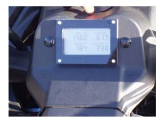
I recently added a graphic LCD screen to my Goldwing. The new screen displays battery voltage, battery current (either charging or discharging), outside temperature, and altitude derived from a pressure sensor. It is also interfaced to an OEM GPS board and displays exact time and date, latitude, longitude, current speed, a resettable odometer, current direction, and altitude derived from the GPS.
