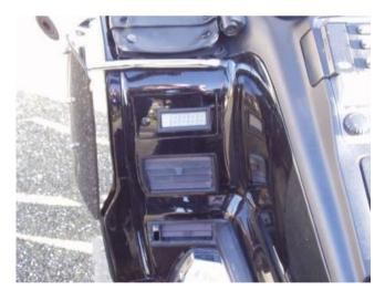
My first attempt was a 5 digit LED display that I mounted in the blank panel where a CB would be mounted since I don't have one on this bike. The voltage worked great, the temperature worked great, the current sensor that I wanted to use was not available yet so I didn't have current sensing yet, and the altitude worked relatively well but could be off by +/- 200 feet or so since it was based on an <u>absolute</u> <u>pressure sensor</u> and could
